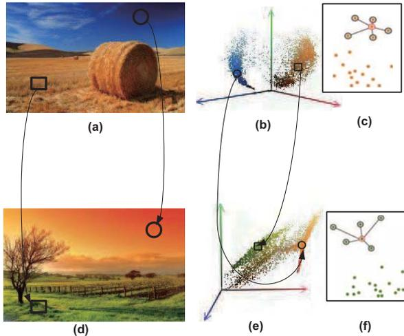
Fig. 5. The illustration of image color clustering and color transfer by CLLE.
