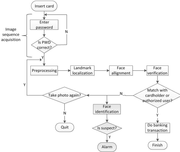
**Fig. 1.** The proposed pipeline of face recognition. The image is acquired at the moment of the card insertion. If current image is matched with card-holder or one of the authorized user’s images, the process is continued. Otherwise, while asking him whether take photo again we can implicitly recognize the current user’s identification to judge whether the user is a suspect, if yes, send alarm signal to monitoring center by background program.
