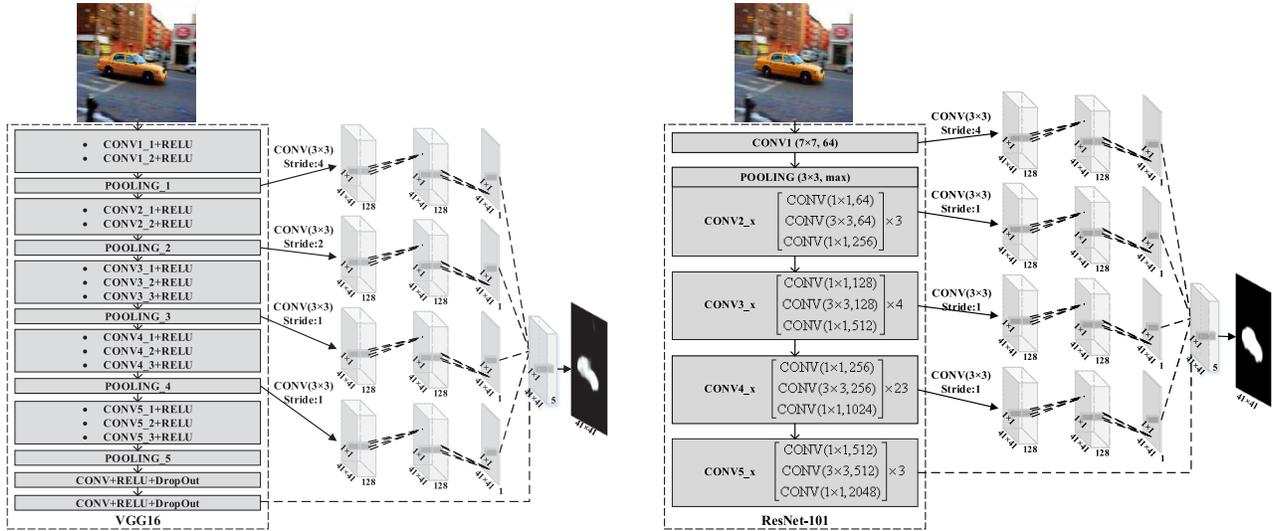
Fig. 2. Architecture of VGG-16-based MS-FCN (left) and ResNet-101-based MS-FCN (right). We connect three extra convolutional layers to each of the first four max-pooling layers of VGG-16 and convert it to a multiscale version. For ResNet-101, we divide the 101 layers into five groups and connect an extra subnetwork with three convolutional layers to each of the final layers in the first four groups to form the multiscale version.
