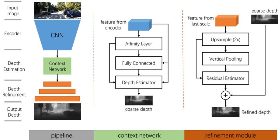
**Fig. 1.** An overview of the proposed network. The network is composed of a deep CNN for encoding image input, a context network for estimating coarse depth, and a multi-scale refinement module to predict more accurate depth. The context network adopts affinity and fully-connected layers to capture neighboring and global context information, respectively. The refinement module upsamples the coarse depth gradually by learning residual maps with features from previous scale and vertical pooling.
