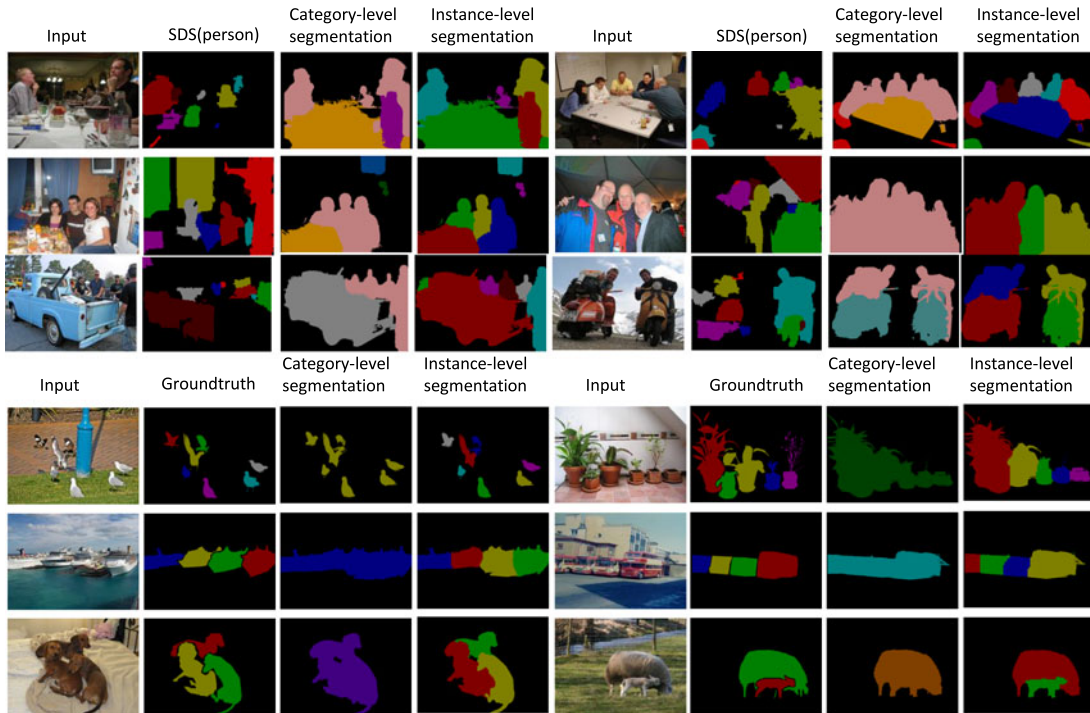
Fig. 6. Illustration of instance-level object segmentation results by the proposed PFN. We also compare our results with that of SDS [39]. Since SDS [39] predicts the scores for each proposal of each category, the top 10 predictions for each image of the person category are shown for the visual comparison. Note that for instance-level segmentation results, different colors only indicate different object instances and do not represent the semantic categories. In terms of category-level segmentation, different colors are used to denote different semantic labels. Best viewed in color.
