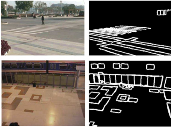
Fig. 10. Sketch detection results refined by Gaussian filtering and edge linking. The primal sketch algorithm [6] is applied to obtain the sketchable regions (light color) and the unsketchable regions (dark color).
