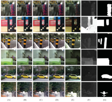
Fig. 3. Examples in the HFUT-Lytro dataset. From (A) to (G): all-in-focus images, focal slices sampled from different depth planes, center viewing images, depth maps, and human-masked ground truths.
