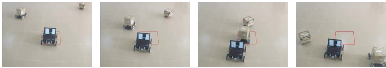
(a) Initial positions of the robot and (b) The robot started to avoid the two obstacles. (c) The robot avoided one obstacle. (d) The robot avoided the two obstacles and started to move back to its initial position.
