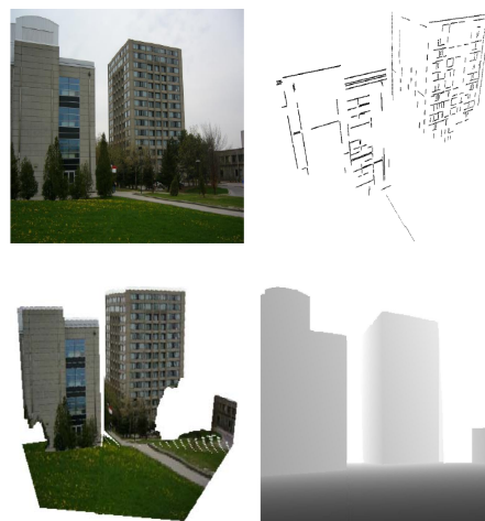
Figure 1: Single-view 3D Scene reconstruction. (a) input image; (b) novel view of 3D lines; (c) novel view of the input image; (d) the recovered depth map.
