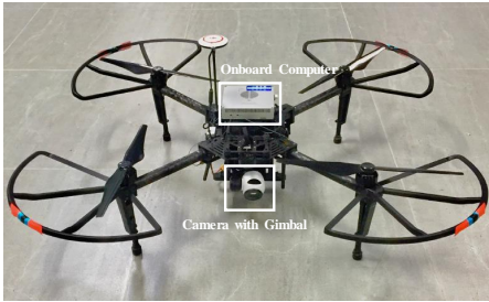
Fig. 7. The experimental test-bed: DJI Matrice 100 UAV with onboard computer and monocular RGB gimbal camera system.
