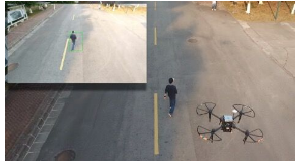
Fig. 1. An instant of our flight experiments. The upper left corner is an image of the onboard camera, where the green rectangle is the bounding box indicating the current state of the target.
